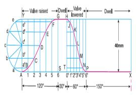
Fig 6: Displacement of CAM
