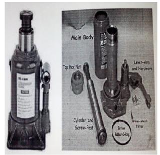
Fig 3: Bottle Hydraulic Jack (Exploded)
